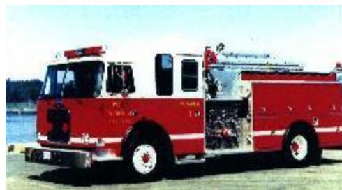
New 1991 1050 gpm GM/White/Volvo Diesel Powered Pumper with enclosed crew cab.
