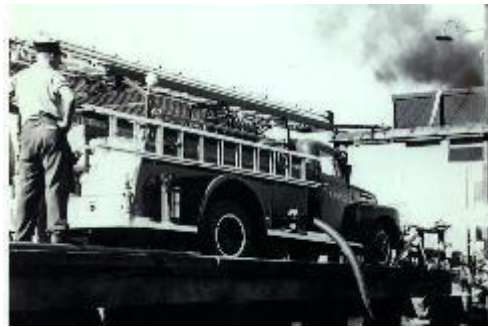
1949 Pumper shown undergoing it's acceptance pumping tests.
