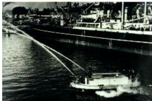
Photograph shows the Port Alberni Fire Department personnel operating the vessel while an engineer from the Provincial Fire Marshal's Office takes readings of water flow to establish the vessel's official pumping capacity.
