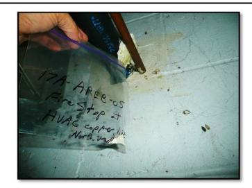
Sample 17A-AREB-05 - fire stop at the copper line on the northeast wall of the AREB was 'none Detected' for asbestos.
