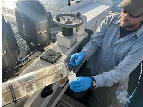
Photo 9. Marine receiving environment water sample collected with Van Dorn grab sampler (September 9, 2024).
