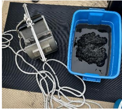
Photo 16. Sediment collected in tote for benthic invertebrate sampling (September 23, 2024).
