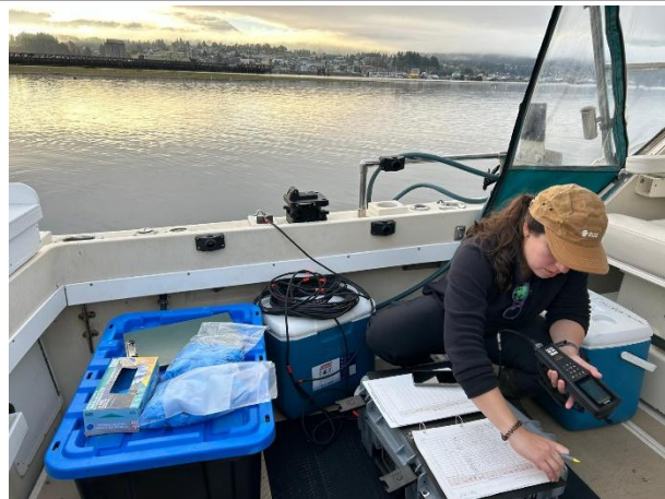
Photo 12. In-situ marine water quality data collected with YSI multi-parameter unit (September 16, 2024).
