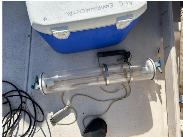
Photo 6. Van Dorn grab sampler used for marine receiving environment sampling (September 3, 2024).
