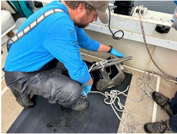
Photo 15. Standard ponar grab sampler used for sediment sampling (September 23, 2024).
