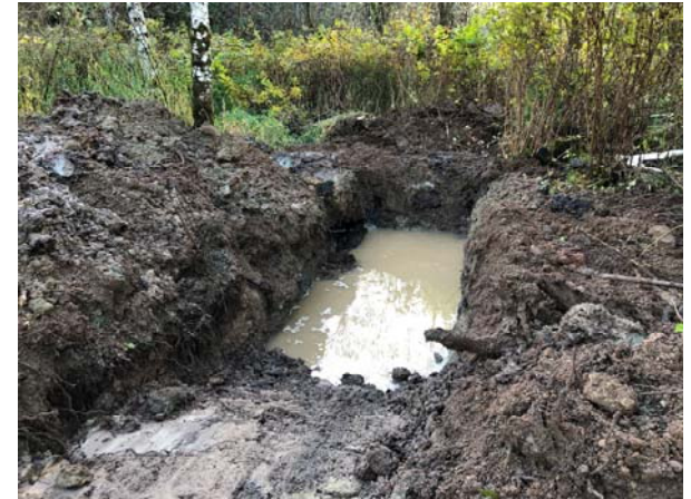
Photo 9. Testpit near the wetland on the west side of tracks showing no sheening or product.
