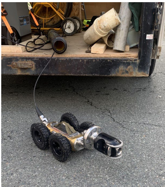
Figure 2: New Sewer Crawler Video Inspection Unit
